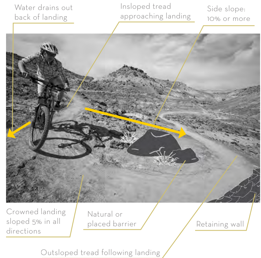
FIGURE 32. Rolled Crown Switchback
